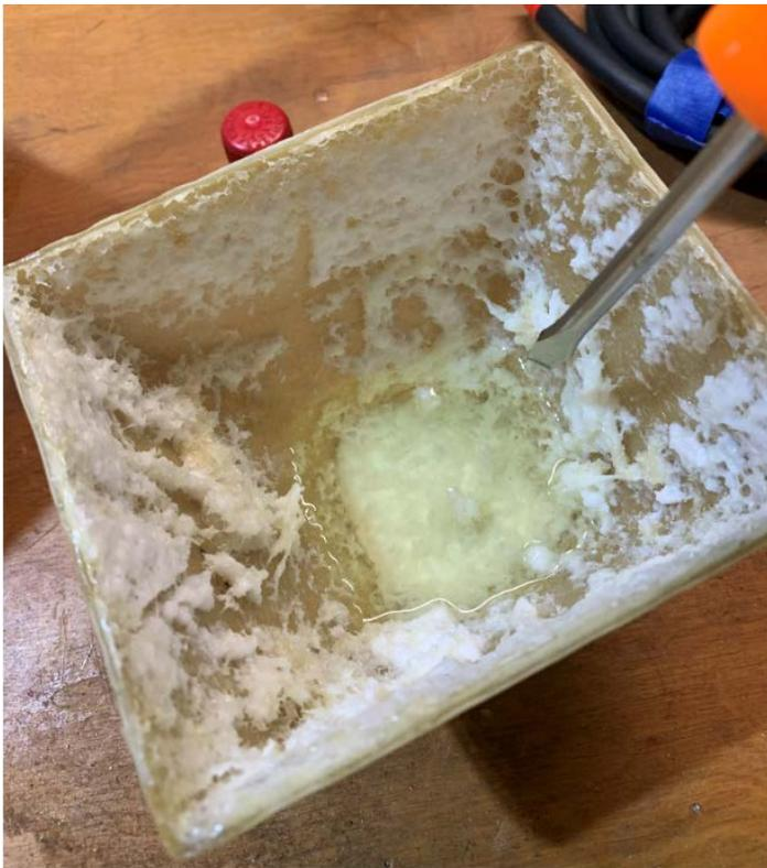
I tipped the cowl around to let the gas get to all areas of the foam. Then scraped with a screw driver to remove the foam slushy
