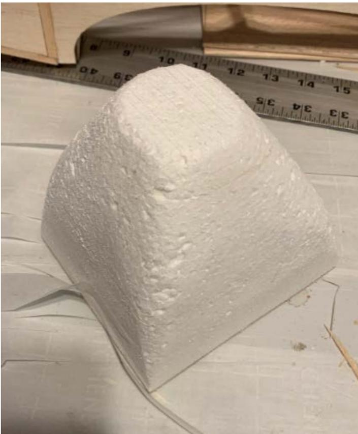
I then smoothed it with 150 grit sandpaper, removed the plywood base and glued four sticks into the bottom to support the form off the working surface.
