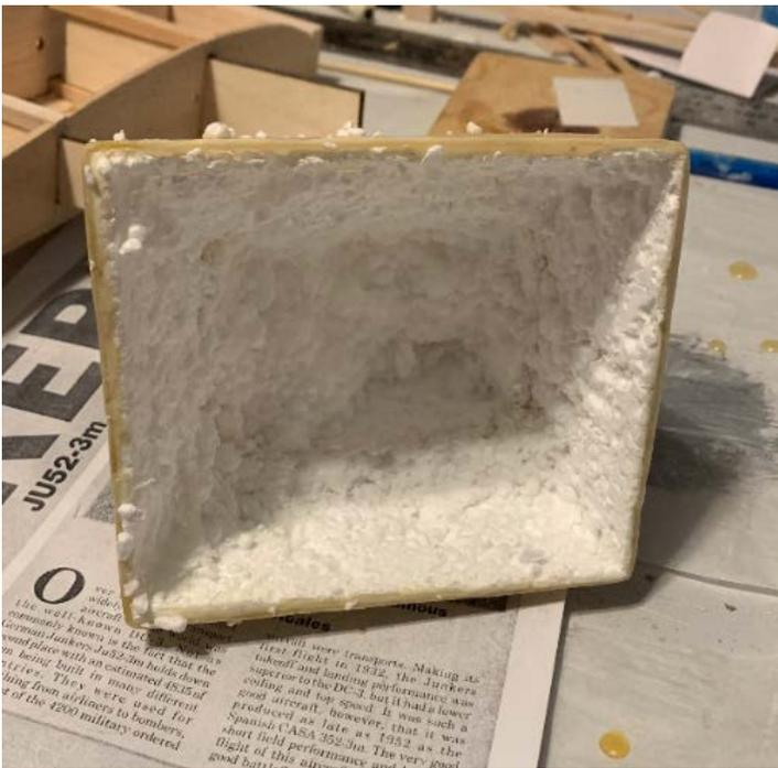
Then about a half of cup of gasoline was used to melt the remaining foam. (Done in a very well ventilated area).
