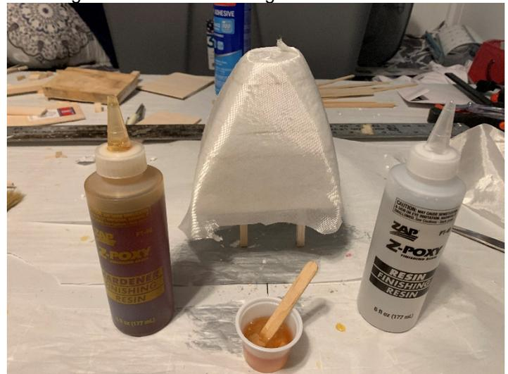
I did Three layers of 1.5oz cloth then the final was .5oz cloth to get a fairly smooth surface, allowing the resin to dry between layers. I did a final layer of resin mixed 50/50 with microballoons which really covered up the weave.
